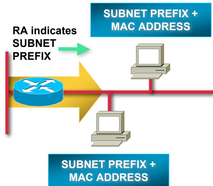
**At boot time, an IPv6 host build a Link-Local address, then its global IPv6 address(es) from RA**
