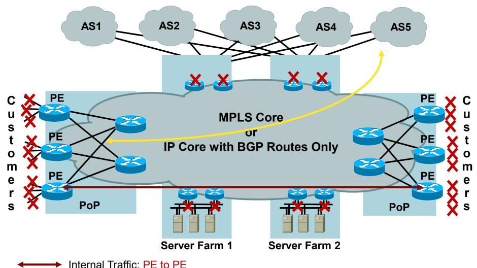
Internal Traffic PE to PE
