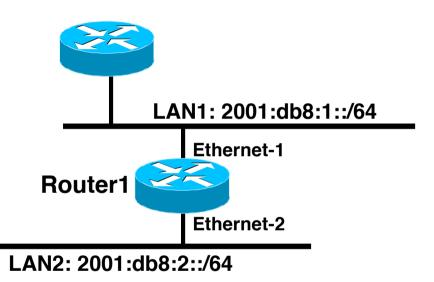
Dual IPv4/IPv6 configuration. Redistributing both IPv6 static routes and IPv4 static routes. Router1# interface ethernet-1 ip address 10.1.1.1 255.255.255.0 ipv6 address 2001:db8:1::1/64 ip router isis ipv6 router isis
