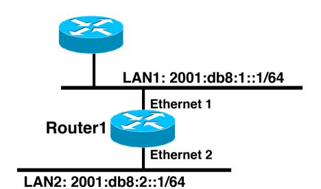
Dual IPv4/IPv6 configuration - note single-topology command —
