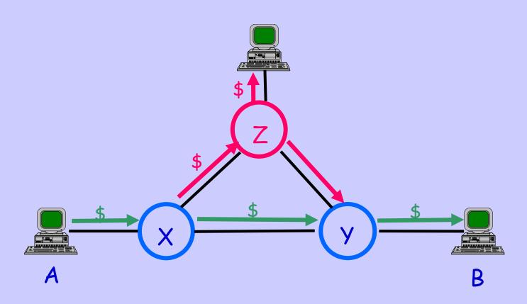
Expected Path - A->X->Y->B Diverted Path - A->X->Z->Y->B
