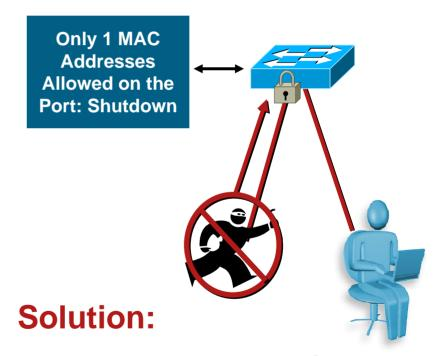
Port security limits MAC flooding attack and locks down port and sends an SNMP trap
