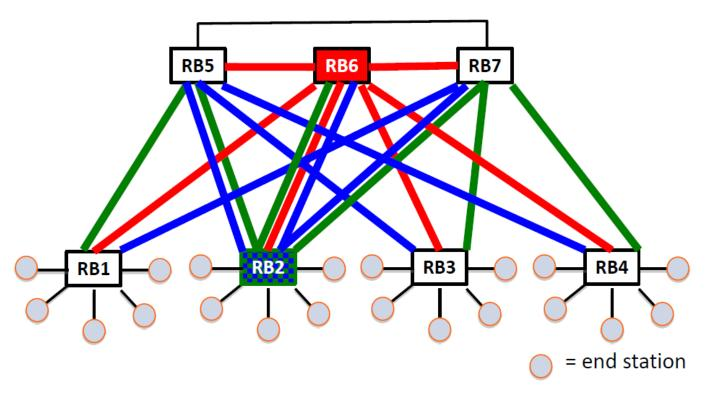
RBridges support multiple distribution trees. The encapsulating Rbridge chooses which to use. RB2 can split multi-destination traffic over three trees.
