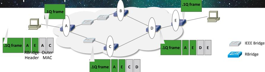
Frames are encapsulated with the RBridge addresses and further encapsulated with originating rbridge and next hop rbridge MAC address
