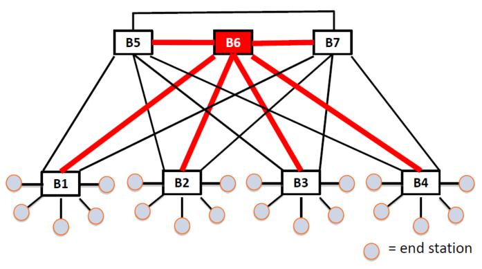
Spanning tree yields a single bi-directional tree for flooding multi-destination frames limiting bandwidth
